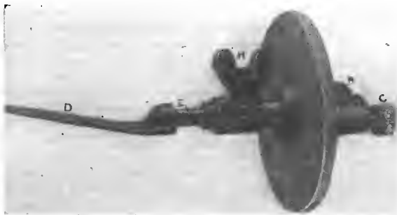
Fig. 2.—Profile view of the Larrad. A, disc; B, spirit level; C, pin; D, blade for attaching; E, shaft to be fixed parallel with the crankshaft; H, winged nut fixing disc A to shaft E.
